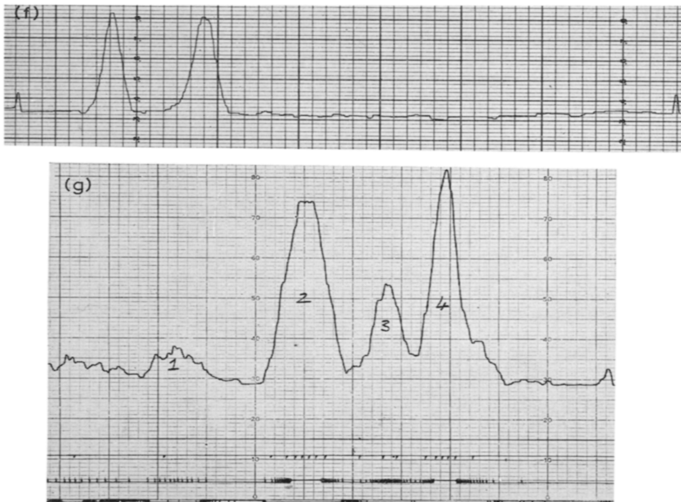
Fig. 7. Scanning records. (f) 25 \mu\text{g} of cortisol (f) and cortisone (E) by the alkaline BT method. Z_1 , o, pencil lines at front and origin respectively. Esterline Angus Labgraph recorder, low sensitivity, minimal damping. Whatman SG81 paper, unwashed. (g) Typical record of the main reducing steroids of human urine using alkaline BT 6 . 1 = Cortisol; 2 = tetrahydrocortisone; 3 = allotetrahydrocortisol; 4 = tetrahydrocortisol. Heathkit EUW-20A recorder with four-pen integrator (see text). Moderate sensitivity, minimal damping.
